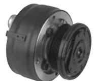
parts of a grenaded compressor into the suction line. This unit uses oil mist lubrication and will NOT TOLERATE ESTER OIL. Use PAG 150 only. Pulley bearing failure on these units is almost always the fault of a seized belt tensioner. Look for other recently replaced parts on the same belt. (alternator, water pump, power steering pump)
