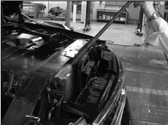
Watch for transmission oil coolers mounted directly onto a condenser. This is a favourite of transmission shops, but the transmission oil is 125C and the condenser is 60C. That means the tranny cooler heats up the condenser. That's the opposite of what a condenser does.
