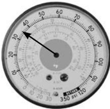
Example: if the system is shut off and temperature is 70F (21C), system pressure would be 74PSI
