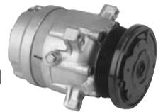
Before condemning this (and other variable displacement compressors), add 100 psi of Nitrogen and turn on the system. A good compressor will pump over 225psi on the high side. Higher pressures indicate a blocked TXV. The low side always stays at 28-35psi. See page 33.
