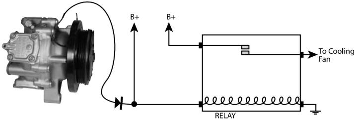
TO MAKE THE ELECTRIC FAN COME ON WITH COMPRESSOR, ADD A WIRE SPICED FROM COMPRESSOR CLUTCH FEED TO HOT SIDE OF FAN RELAY COIL.
