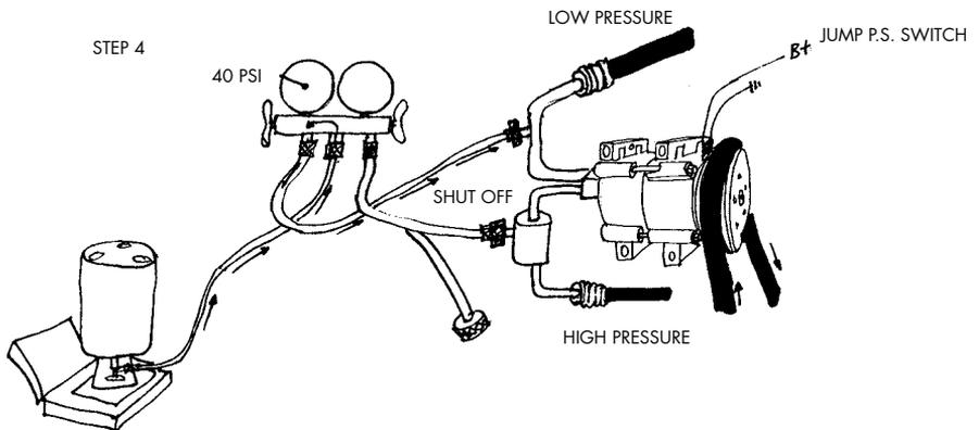
BEFORE USING ANY RECYCLED REFRIGERANT, CHECK ITS PRESSURE!
